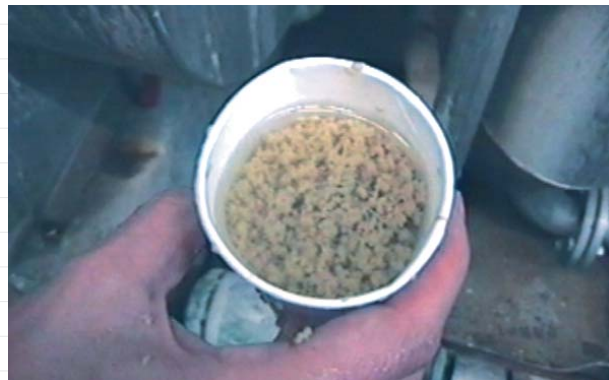
The bio-sludge after flocculation and before filtering
