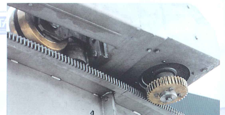
Bridge drive by gear pinion (without security protection)
